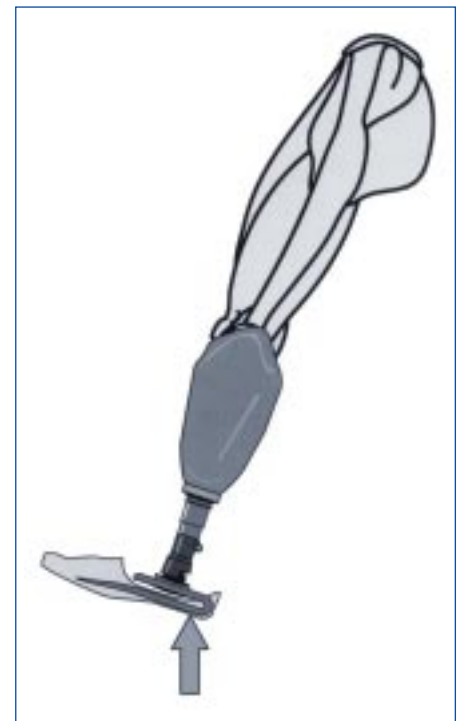
Fig. 2 The socket is responsible for body weight containment during stance phase and for transferring the forces through the components into the ground.
