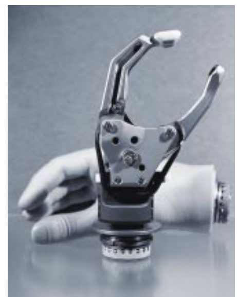
Fig. 1 Sensor hand with automatic grip stabilizer.
