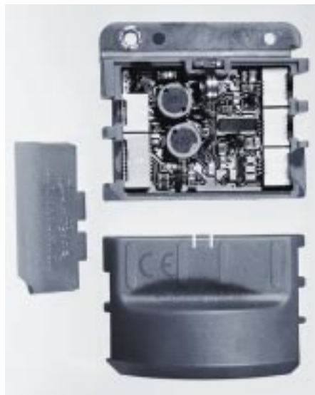
Fig. 15 Miniaturized electronic control unit, programmed via code-plug.
