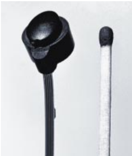
Fig. 11 Modular exchangeable miniaturized "gliding sensor". For size comparison a match alongside.
