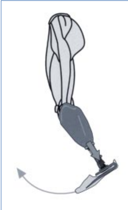
Fig. 3 This gives an example of the connection between a silicone socket and the residual limb.
