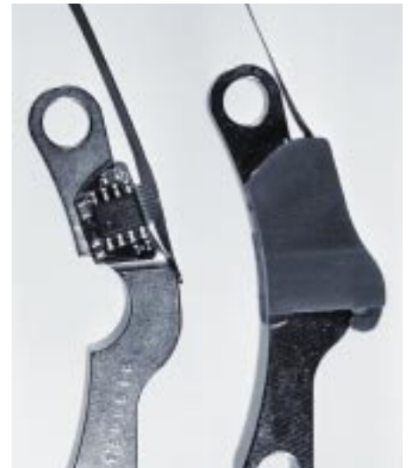
Fig. 13 "Finger stirrup with sensor" used for measuring of the gripping force between thumb and fingers.
